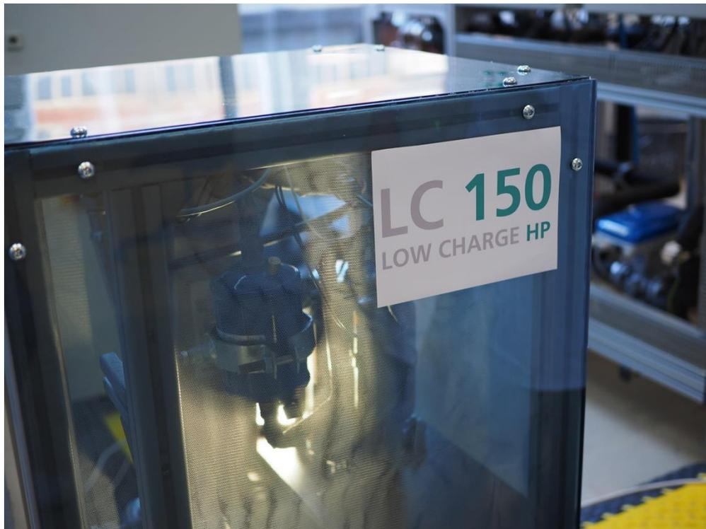
Efficient heat pump using the climate-friendly refrigerant propane developed at Fraunhofer ISE for indoor installations. ©Fraunhofer ISE
