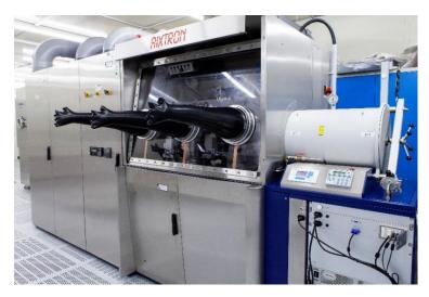
The MOCVD system of Fraunhofer IAF has been modified by the research group to enable the growth of AlScN with sufficient quality and productivity for industry.
