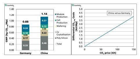
Carbon footprint of a Cz PERC glass-backsheet module production (left). Delta CO<sub>2</sub> cost of a Cz PERC module production located in Germany compared to China (right). Source: own calculations.
