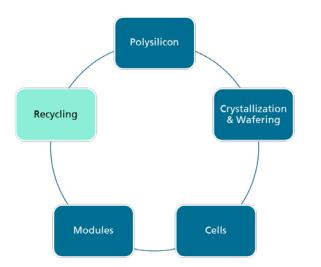
At the end of the life cycle nearly 100 % of the parts of a module will be made available for a new life cycle. The cost for the recycling process must be considered at the beginning of the cycles.
