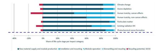
Life cycle analyzes carried out for PV installations highlight the potential for more sustainable PV production and installation. The graph clearly shows that the greatest potential for all Product Environmental Footprint Category (PEFCs) lies in material flow and production towards the module (see also: http://www.etippv.eu/fileadmin/Documents/ETIP PV Publications 2017-2018/181122 -ETIP PV Report on PV Quality and Economy web.pdf)
