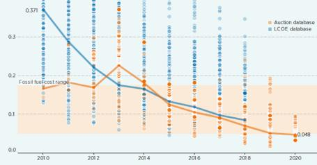
Levelized Costs of Electricity (LCOE) in US\$/kWh for solar PV projects. Source: Future of Solar Photovoltaics, Report, IRENA, 2019
