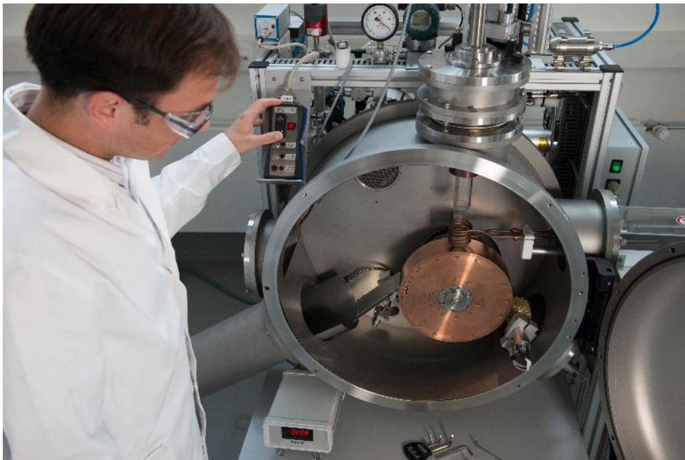
Melt-spinner at the technical center of Fraunhofer IWKS. © Fraunhofer IWKS
