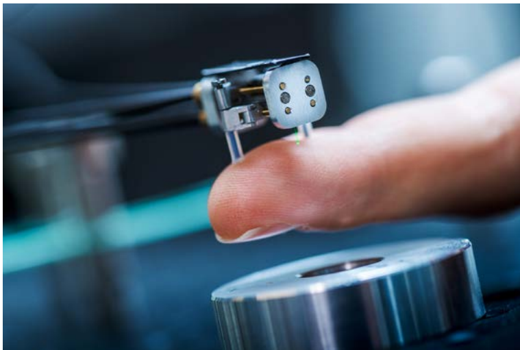
01: One of the results of the first funding phase: a high-precision robot endoscope tip with integrated laser bone saw. Picture: Werner Siemens-Stiftung, F. Brüderli
