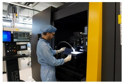
Fully automated roll-to-roll laser transfer and firing system at Fraunhofer ISE. The system was developed within the collaborative project "C3PO", which was financed by German federal and state funds.
