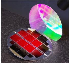
The new III-V//Si tandem solar cell with 35.9 % efficiency. The top subcell glows red, which is a sign of outstanding material quality. The nanostructured back side of the cell shimmers in rainbow colors. © Fraunhofer ISE / Photo: Michael Schachtner **PRESS RELEASE** April 23, 2021 || Page 2 | 3
