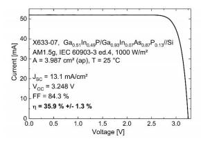
I-V characteristic of the new III-V//Si triple-junction solar cell, measured at Fraunhofer ISE CalLab PV Cells. © Fraunhofer ISE
