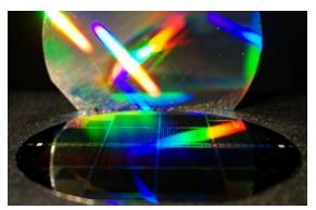
The rainbow colors show the diffraction of sunlight by a mirror with a nanostructured grating, which was applied to the back of the silicon subcell. The sun's spectrum is thus captured even better in the silicon bottom cell. © Fraunhofer ISE / Photo: Michael Schachtner
