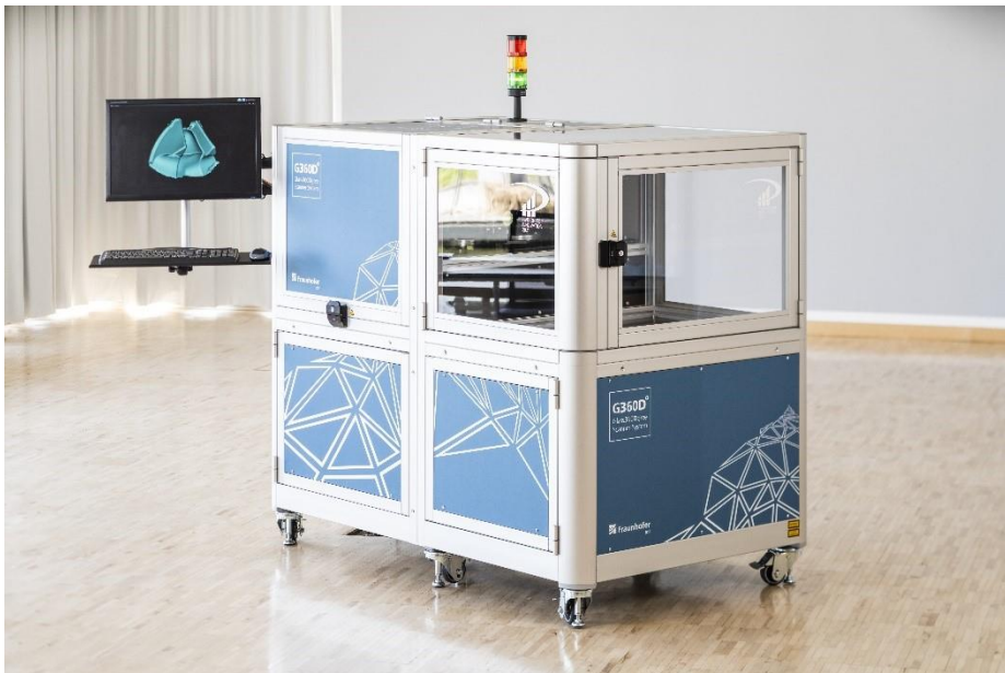
Fig. 2: "Glass360Dgree": First MWIR 3D system for the inspection of glass bodies in optics manufacturing (Copyright: Fraunhofer IOF)
