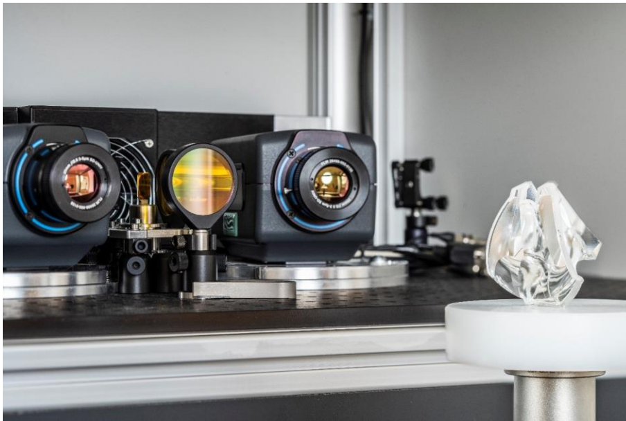
Fig. 5: The system uses thermal radiation for 3D detection of transparent objects (Copyright: Fraunhofer IOF)
