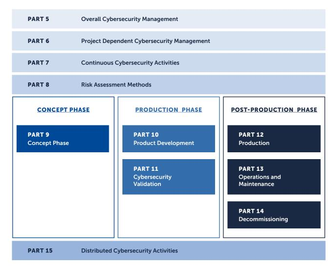
Figure 1. Technical parts of the ISO 21434.
