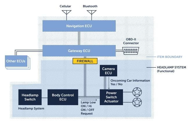
Figure 5. Headlamp system with a Firewall
