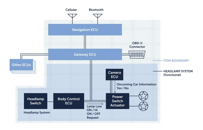
Figure 2. Preliminary architecture of the headlamp system [3]
