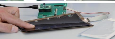
Sensor array and extended CMS circuit for measuring and evaluating the sensor signals. The sensor array measures the deformation of the battery during cycling. © K. Selsam, Fraunhofer ISC
