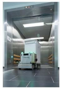
When the robot is linked to the elevator control system, it can move freely around the building.
