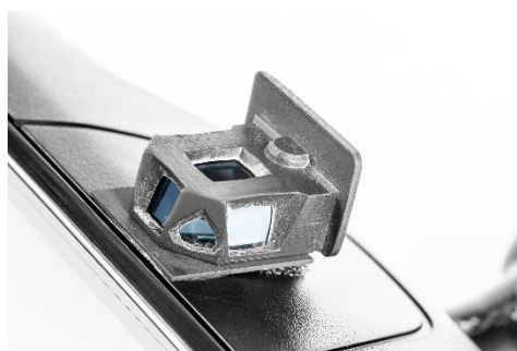
Fig. 3: The miniaturized wide-angle 3D camera is mounted on the bottom of the rearview mirror. Shown here in close-up. © Fraunhofer IOF
