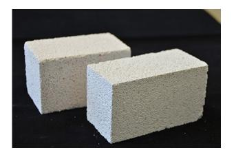
The climate-friendly aerated concrete scores with its excellent insulating properties, long service life and good acoustic properties.
