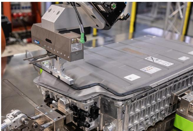
**The project developed a variety of hardware for automated disassembly tasks, such as this small parts gripper.**
