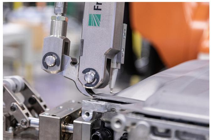
**A tool dubbed "Knacker" was developed to prize apart the adhesive bonds between the upper and lower shell of a battery.**
