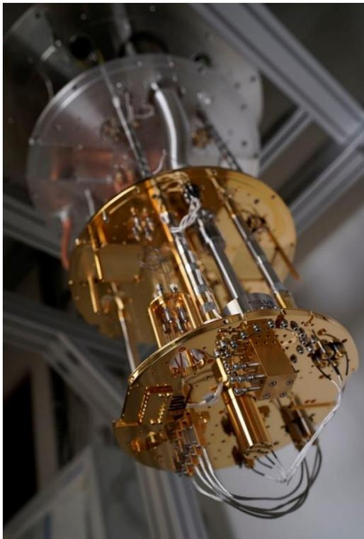
1 K cryostat with conducted lines for direct current and high-frequency measurements,
