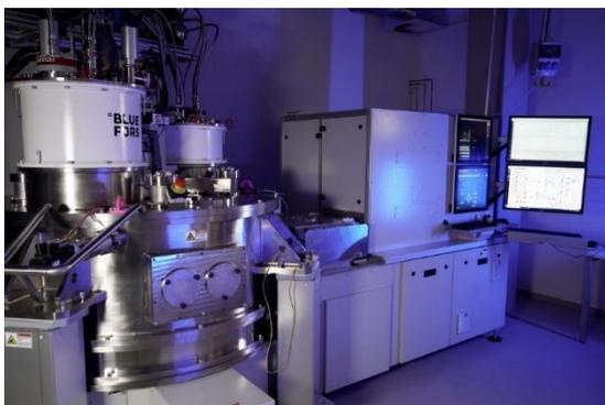
The cryogenic on-wafer prober at Fraunhofer IAF enables fully automatic characterizations of up to 25 whole 200-mm or 300-mm wafers with devices for quantum computing and sensing.
