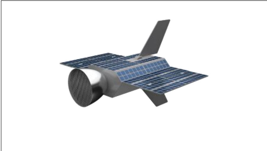
Fictitious representation of a VLEO satellite: This illustrates some of the components and subsystems developed by the ATLAS CRC. Photo: CRC ATLAS
