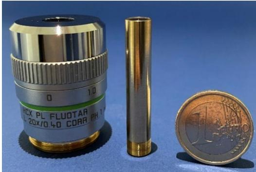
The diameter of a single ComplexEye lens (photo: centre) is 8 mm. It fits exactly under one 9 mm cavity of a standard 96 well plate. In a 384 well plate, cavities have a diameter of 4.5 mm. One ComplexEye lens is therefore many times more delicate and yet almost as capable as the 28.5-mm objective (left) of a conventional microscope. (UDE / Prof Dr Matthias Gunzer)
