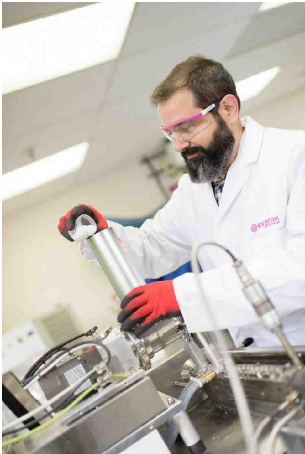
In the Medical Devices Project House in Birmingham (Alabama, USA) Evonik is developing improved materials for medical devices. The photo shows an employee filling an extruder with polymer granulate. Evonik Industries AG
