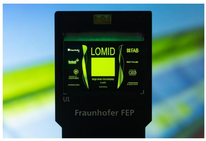
Test and qualification vehicle of the LOMID chip with a screen diagonal of 2.5 cm and a resolution of  $1920 \times 1200$  (WUXGA)
