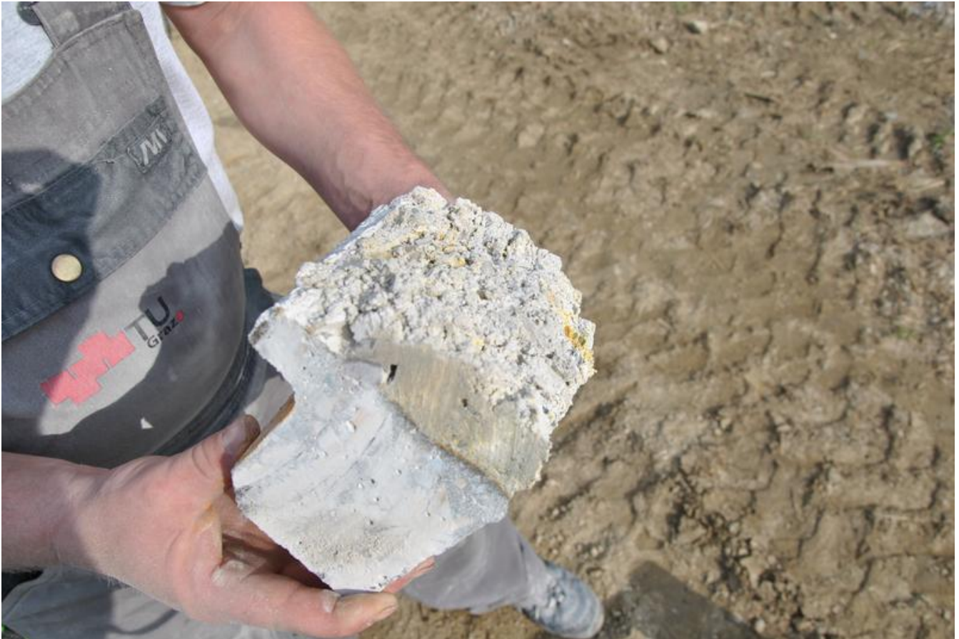
Microbial induced concrete corrosion (MICC) causes massive damage to wastewater plants. Researchers from Graz present a new solution against the sulphuric acid attack. © TU Graz
