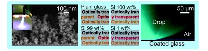
FLTR: Coating by liquid flame spray; surface SEM; letters on paper below liquid repellent coating; confocal microscopy image of water drop resting on coating on glass.
