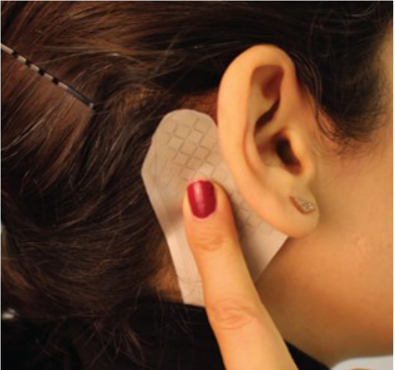
Saarbrücken computer scientists have developed novel skin sensors that allow mobile devices to be controlled from any point on the body. Universität des Saarlandes
