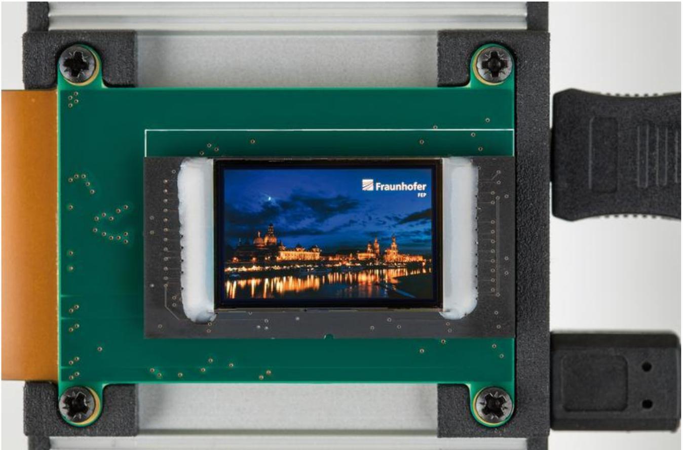
24 mm 120 Hz WUXGA OLED Microdisplay
