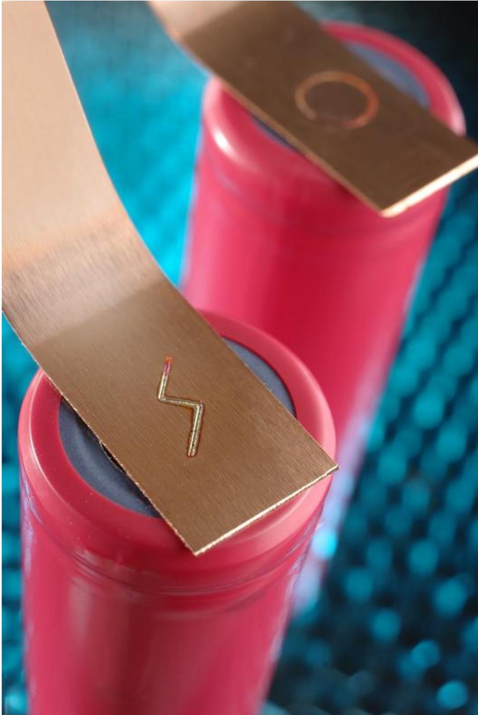
Laser-Based Tape-Automated Bonding (LaserTAB) for the welding of battery cells.
