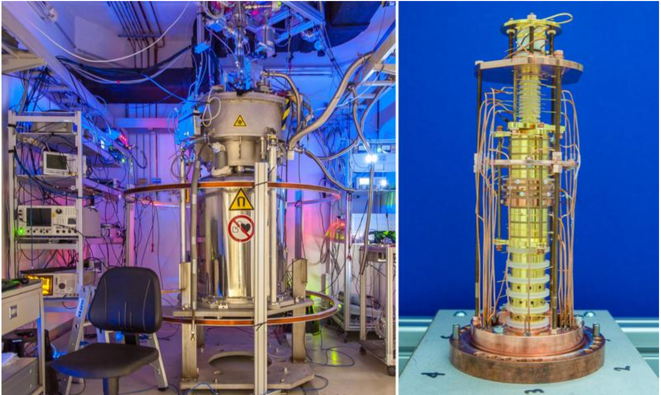
Fig. 1: Alphatrap: on the left the superconducting magnet, on the right the ion trap built into it. Photo: MPIK
