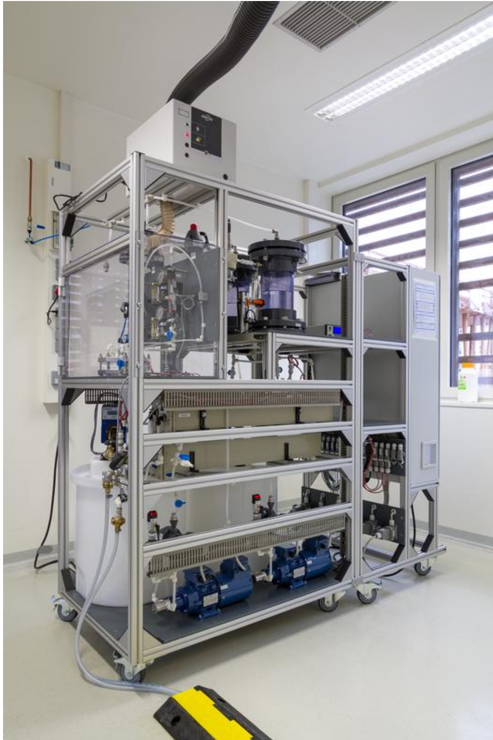
The electrolyzer developed in the CELBICON project at Fraunhofer IGB synthesizes formic acid from atmospheric CO 2 . Fraunhofer IGB
