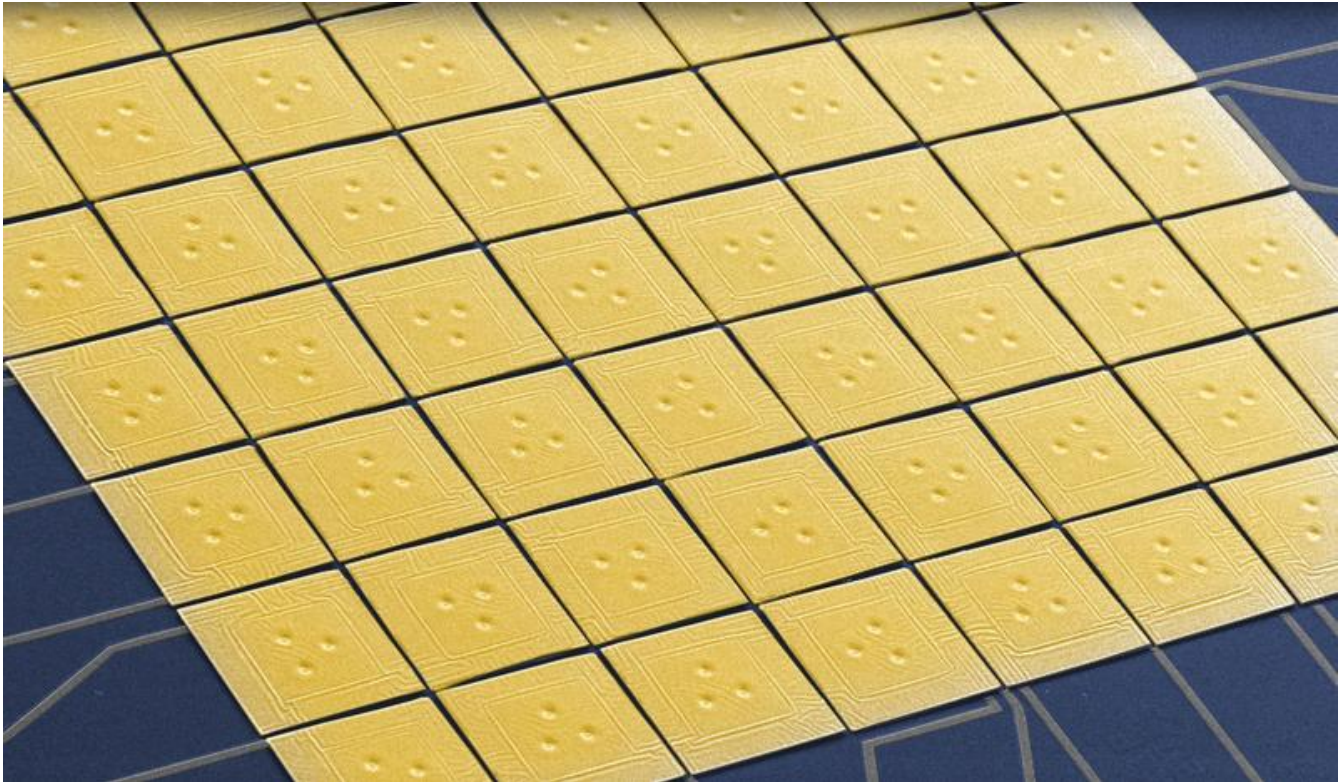
A false color scanning electron microscopy image of the 8x8 array of maXs30 detectors. photo/©: Matthäus Krantz
