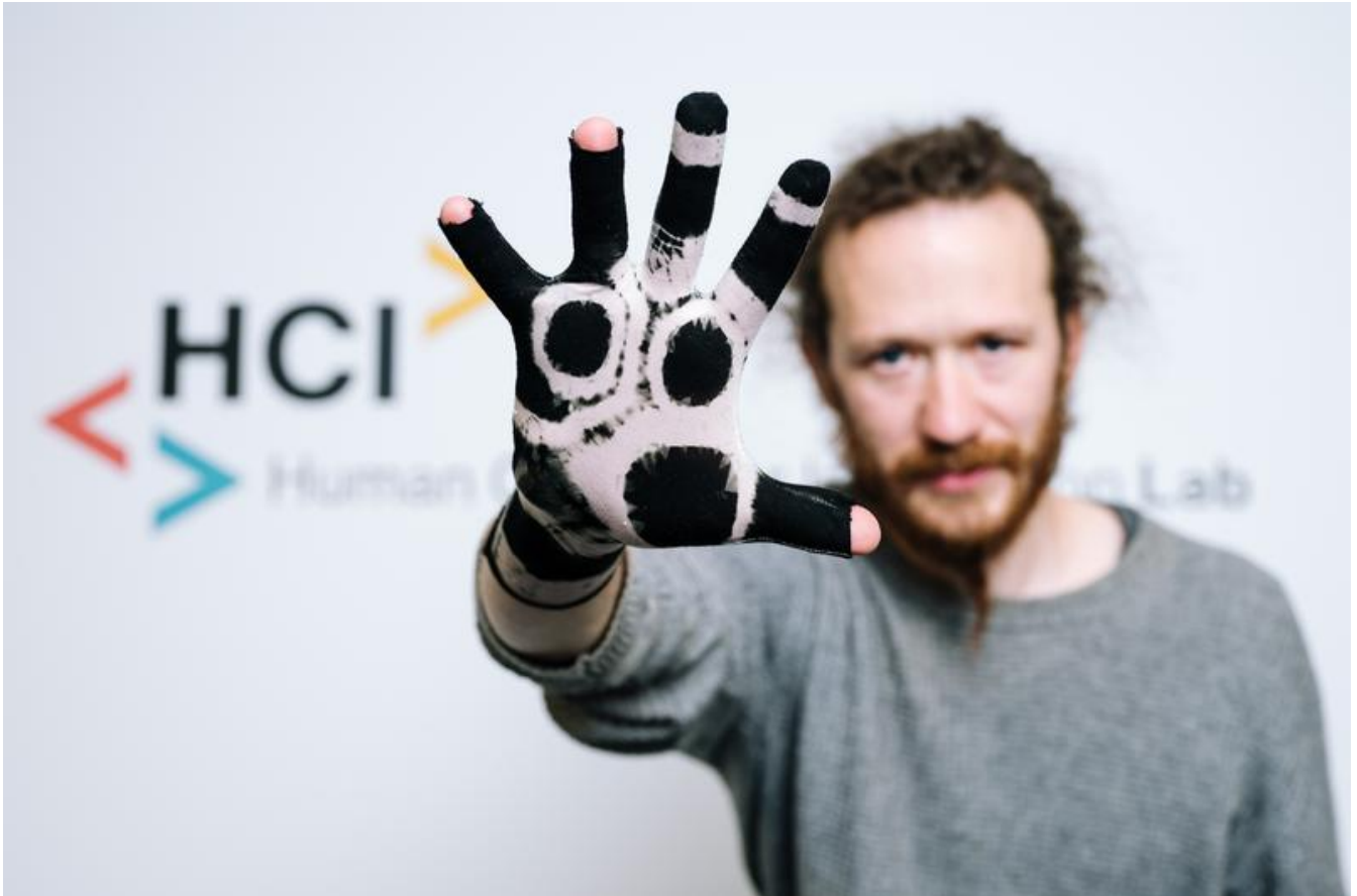
Polymerized glove that can be used to digitally capture hand movements. Oliver Dietze Universität des Saarlandes
