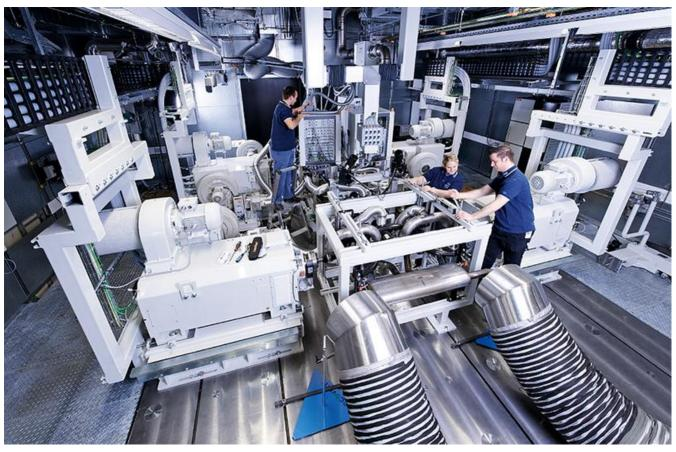
The results from vehicle and engine simulation as well as the influence of carbon-neutral fuels on engine behaviour are tested on a single-cylinder research engine.
