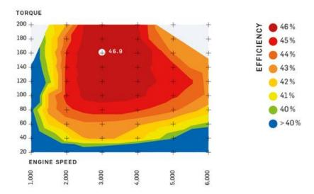
In methanol operation, the new ultimate efficiency engine achieves an efficiency of at least 40% over almost the entire engine characteristic map. vka / RWTH Aachen
