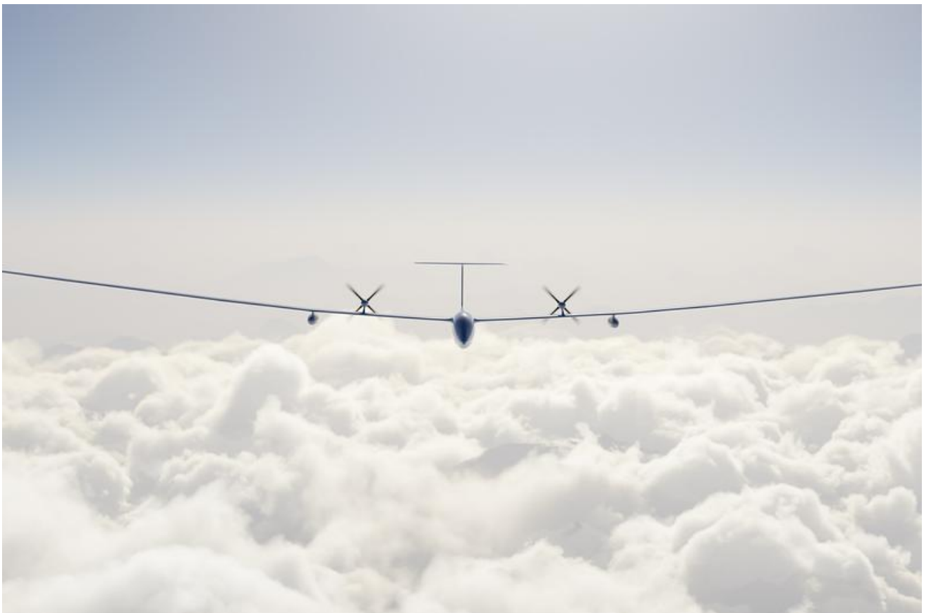
Concept of a Stratospheric Aircraft/High Altitude Pseudo Satellite, or HAPS. Image credits: Leichtwerk Research GmbH
