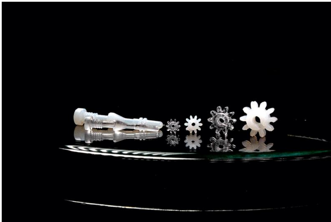
Injection-molded structures made from the newly developed Glassomer composite Photo: Neptun Lab/University of Freiburg
