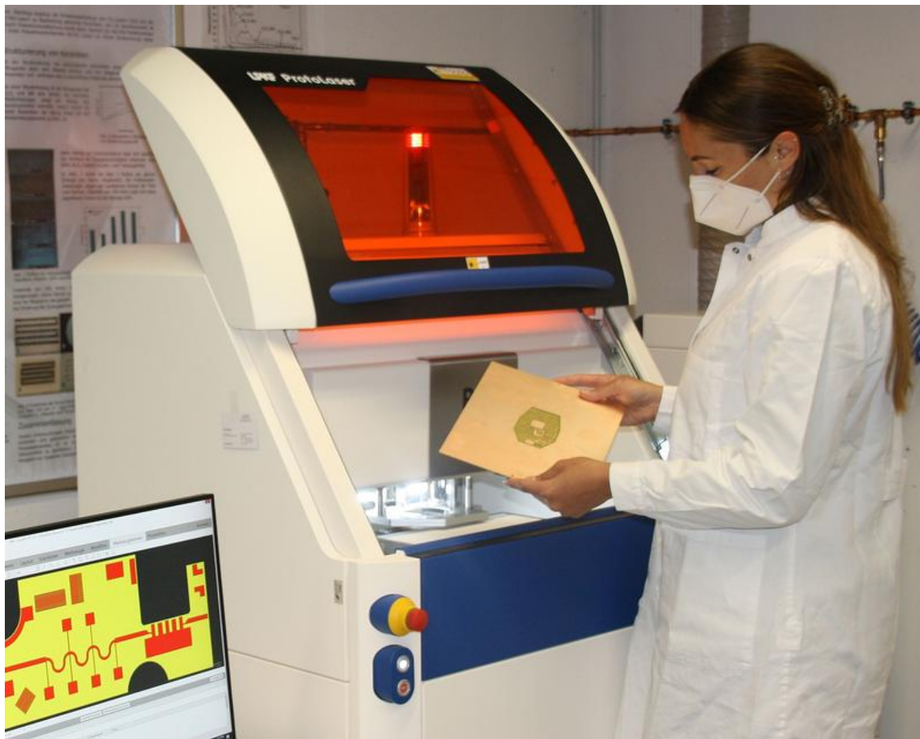
Ultra-fine structuring of a printed circuit board. Photo: C. Wißler.
