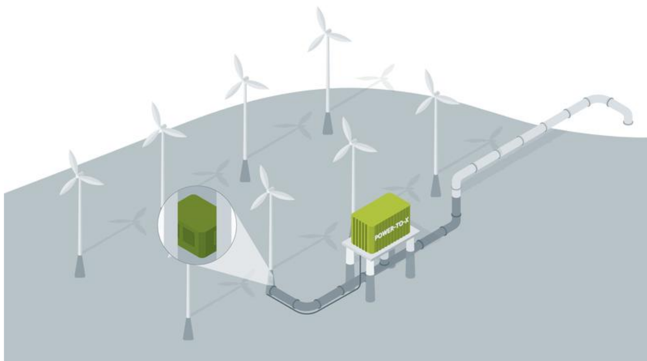
Schematic representation of the offshore production of green hydrogen within the flagship project H2Mare. Project Management Jülich on behalf of the BMBF
