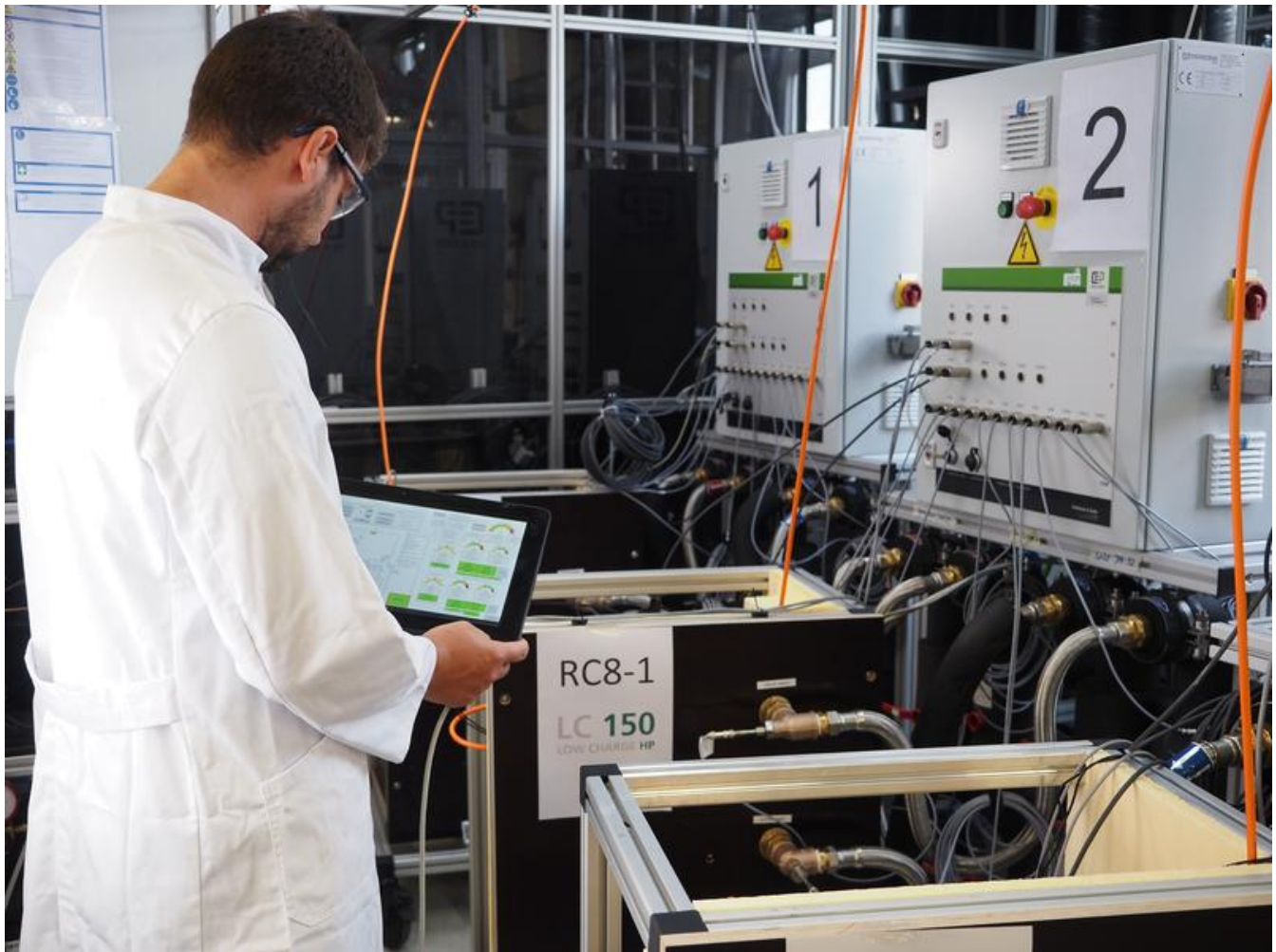
In the measurement campaign, dozens of heat pump component combinations are tested under different operating parameters Fraunhofer ISE
