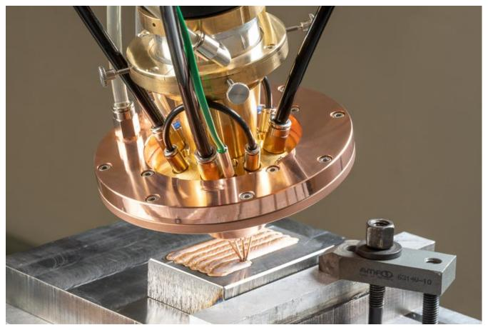
For the first time, simultaneous processing of powder and wire in various combinations becomes possible thanks to COAXquattro.
