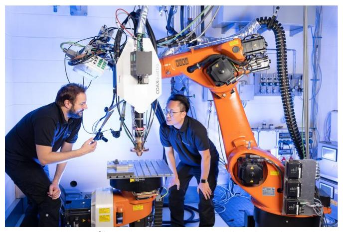
One core element of the HICLAD® family is the innovative COAXquattro laser cladding head. A laser beam runs through the center of the nozzle, around which up to eight separately controllable channels feed wires and powders. © ronaldbonss.com/Fraunhofer IWS
