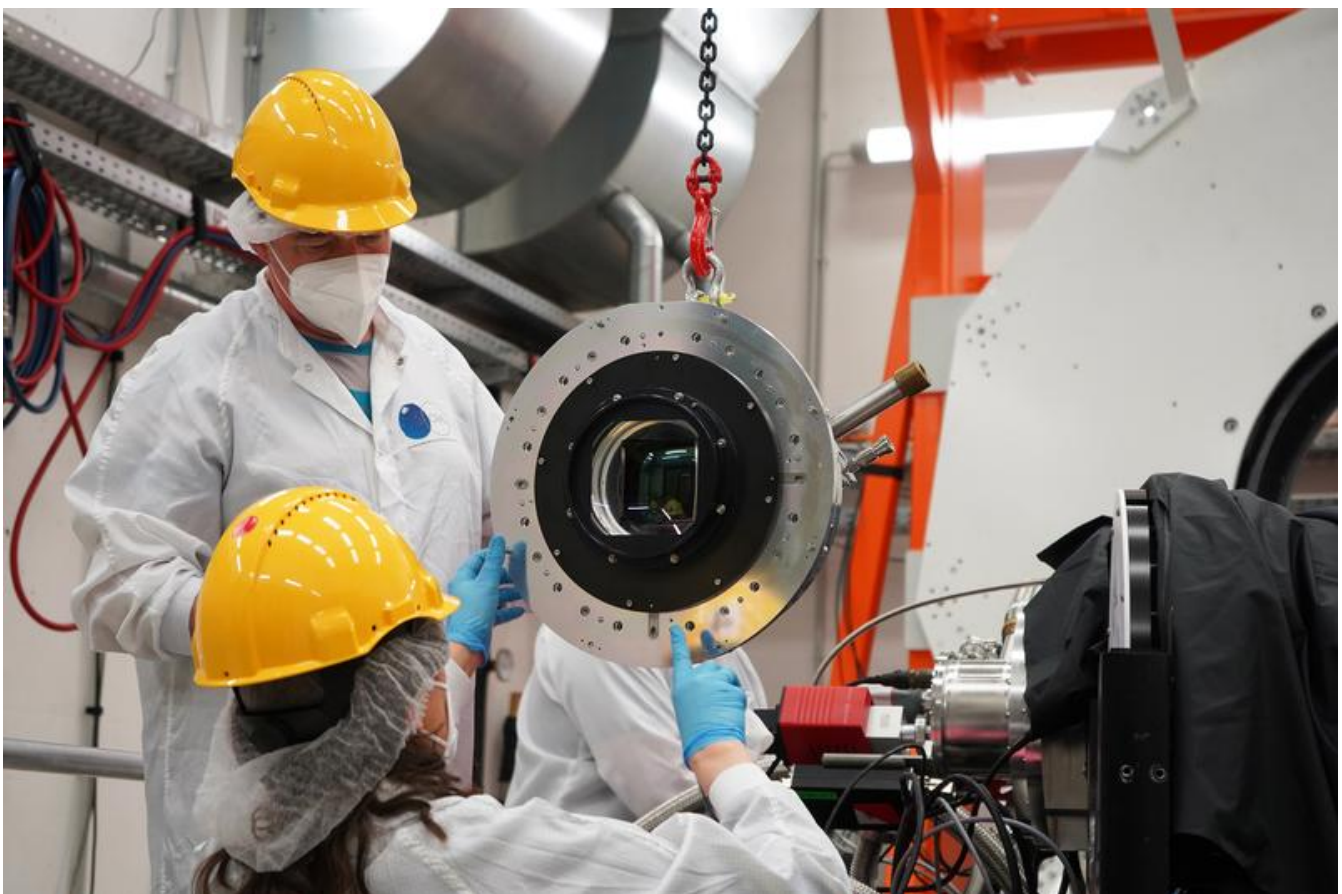
The team installs the detector on the red arm of the spectrograph in the integration hall of AIP. AIP
