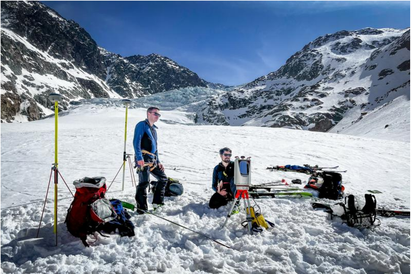
High-tech meets high altitude: Fabian Fleischer and Jakob Rom with laser scanner and GPS antennas below the icefall in the Gepatschferner Glacier PD Dr Florian Haas PD Dr Florian Haas
