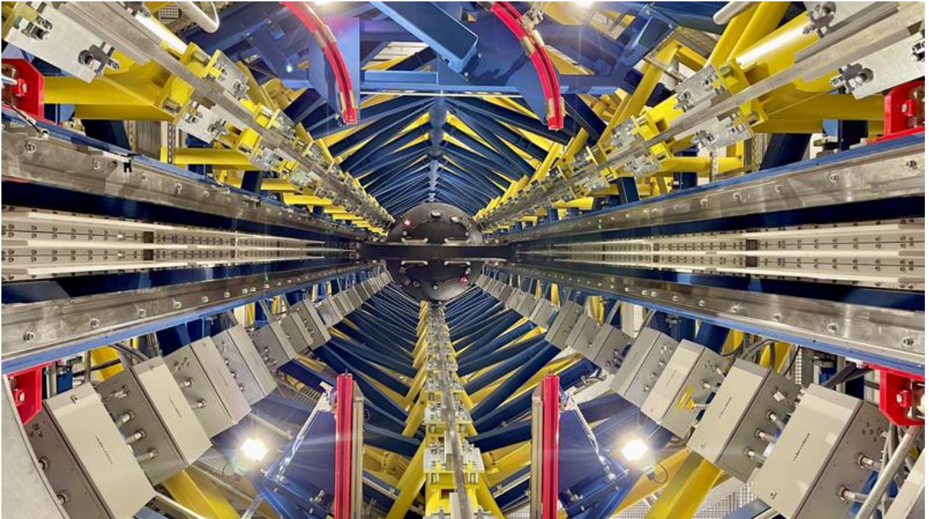
In the Einstein Elevator of Leibniz Universität Hannover, the experiments on welding under microgravity take place. Photo: LUH/Christoph Lotz
