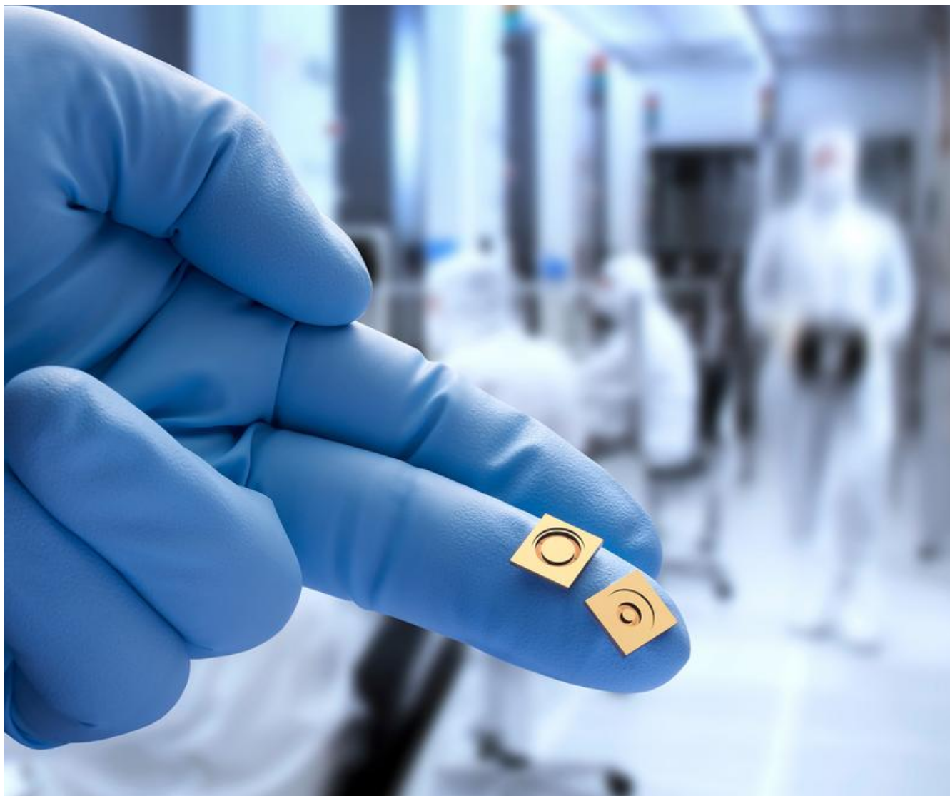
Quasi-static MEMS micro mirrors for LiDAR systems from Fraunhofer ISIT Bodo Schmidt Fraunhofer ISIT / photoccompany Itzehoe
