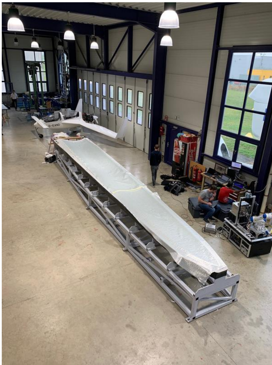
Rotor blade tip with the fiber layer package laid out at Aeroconcept GmbH. © Fraunhofer FHR/André Froehly
