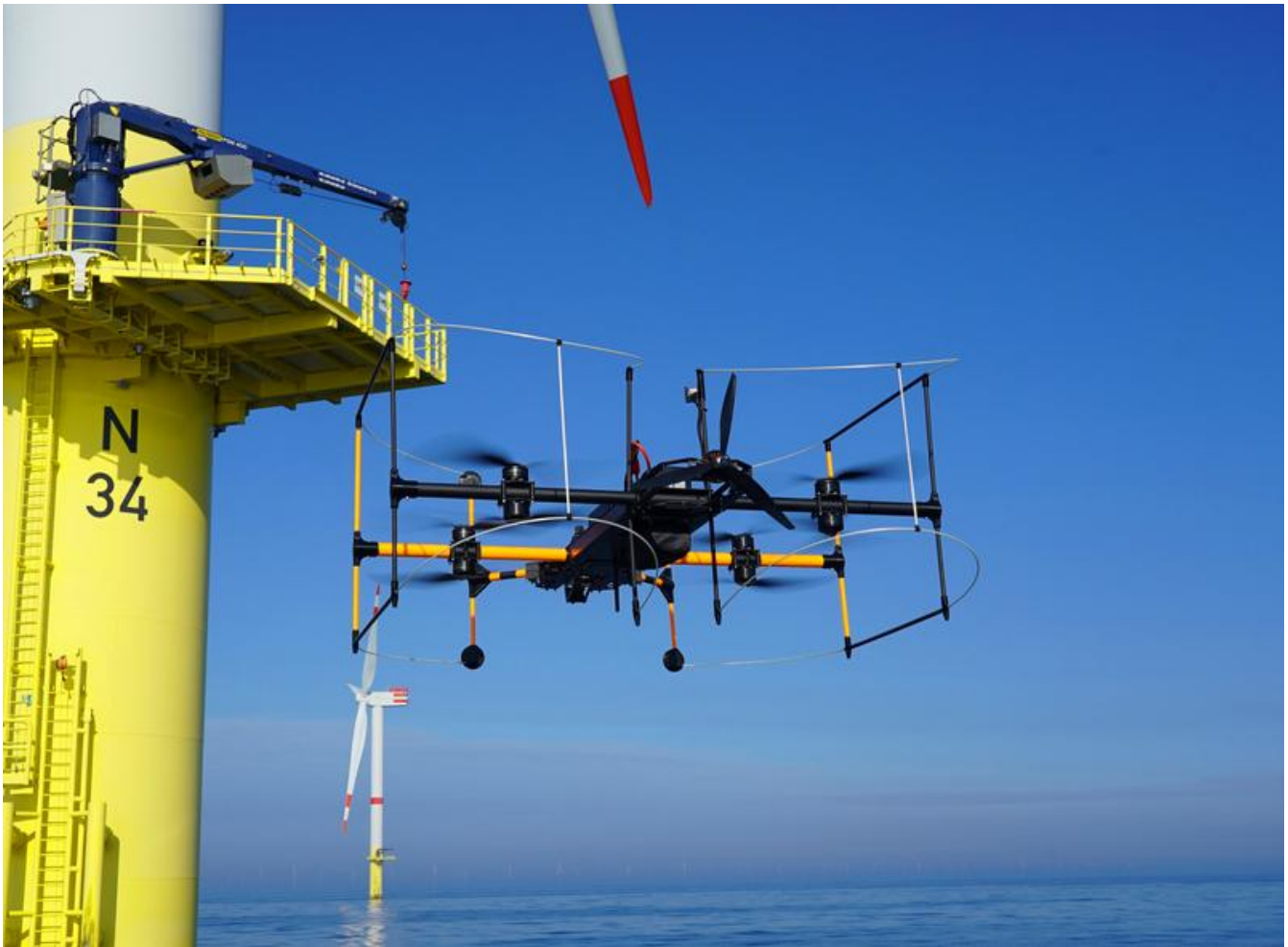
UAS deployment for the inspection of an offshore wind turbine as part of the research project AIDA. Supported by the Federal Ministry for Economic Affairs and Climate Action on the basis of a decision by the German Bundestag, Grant: 03EE3057A. © Fraunhofer IFAM
