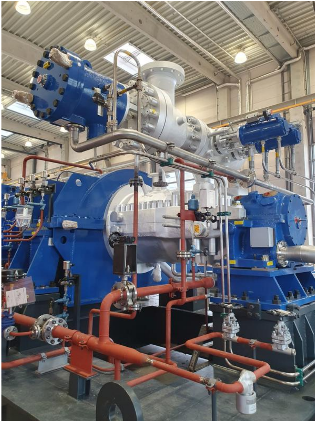
Steam reaction turbine of TGM Kanis Turbinen GmbH with an output of up to 10 MWel.
