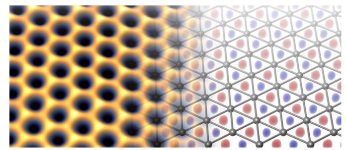
Indene – a topological insulator. The left side shows a measurement of the density of states by scanning tunneling spectroscopy and the right side a schematic representation of the charge distribution in the triangular lattice. CRC ToCoTronics University of Würzburg
