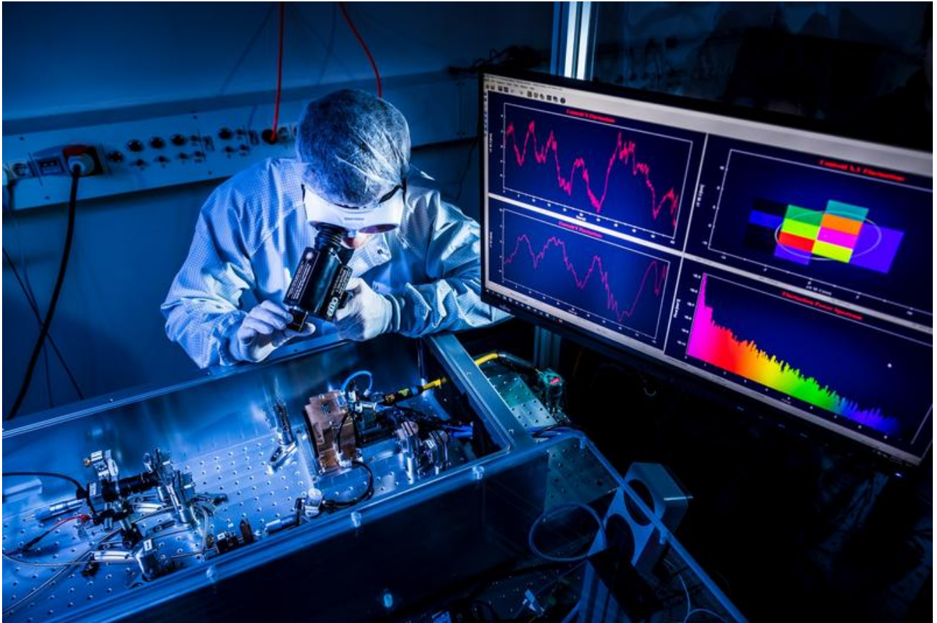
The thin disc laser in its monolithic box leads to operational stability and reproducibility Eric Schambroon Eric Schambroon
