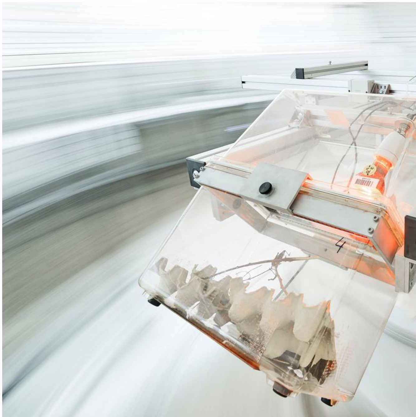
Photo of custom-made centrifuge showing the insect cages with individual heating and LED lighting. Marcus Meyer Photography
