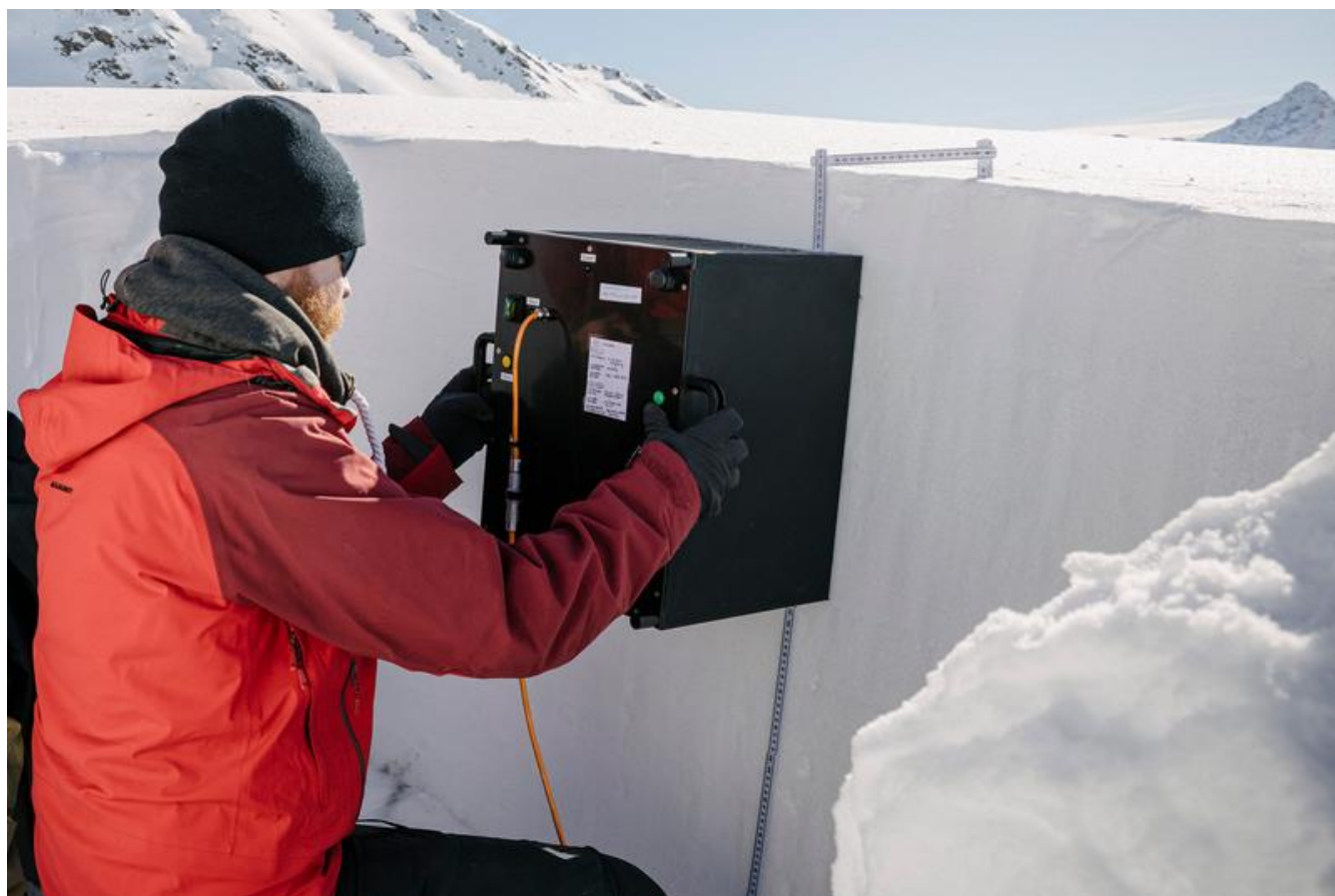
SLF physicist Lars Mewes uses the SnowImager prototype to measure the structure of the snowpack at the Pischascha resort, Davos (Switzerland).
