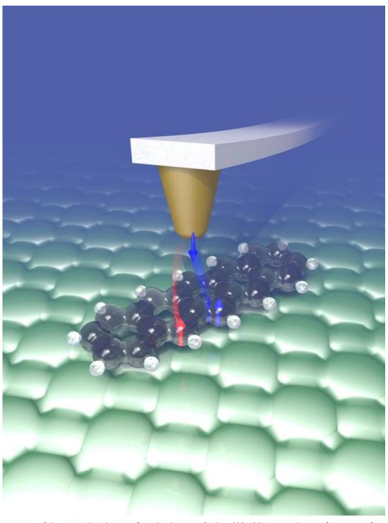
Artistic illustration of the steered exchange of single electrons (red and blue) between the tip of an atomic force microscope (golden) and a single pentacene molecule (black/white spheres) adsorbed on NaCl (green).
