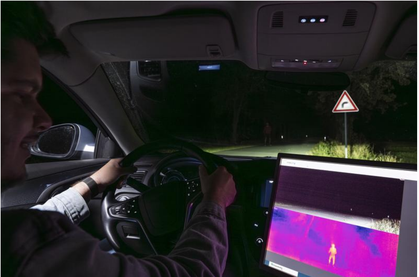
The camera in action: Despite the headlights, the pedestrian at the side of the road is barely visible. Only the thermal imaging camera makes him clearly visible. Fraunhofer IOF
