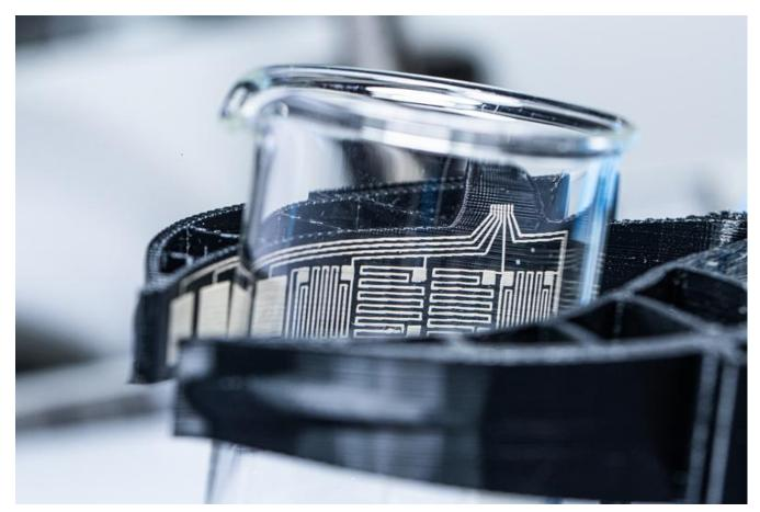
Holds the measuring cup sensitively instead of breaking it: The integrated sensors of the BioGrip grippers can be seen through the glass.
