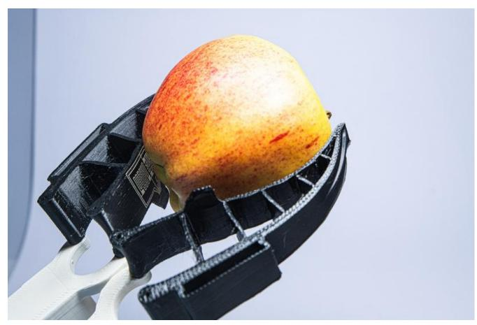
In future, robotic grippers with haptic capabilities will be able to grab and sort apples and other fruit more gently. The gripper developed in the BioGrip project adapts to the apple's shape. © Christoph Wilsnack/Fraunhofer IWS
