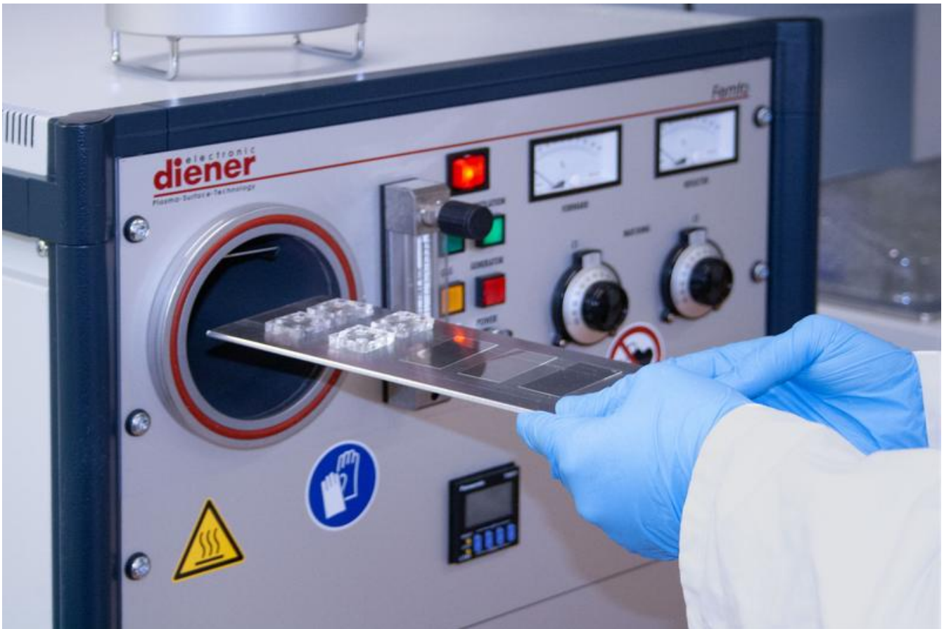
Plasma cleaning step for the production of microfluidic chambers photo/@: Doris Franke / JGU
